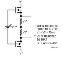
Figure 2. LT1166 Current-Control Loop
